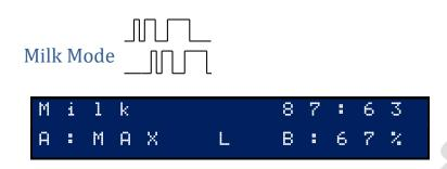
The pulse rate increases and then drops to 0 (continuous). This is similar to Squeeze, but channels A and B alternate. The adjustment control controls how fact the pulse rate goes up or down. The adjustment control controls how fast the pulse rate goes up or down with values from 10 to 100. The second value, is the pulse feel, that allows you to adjust the sensation of each individual pulse, from soft to spiky, with values from 1 to 100.
