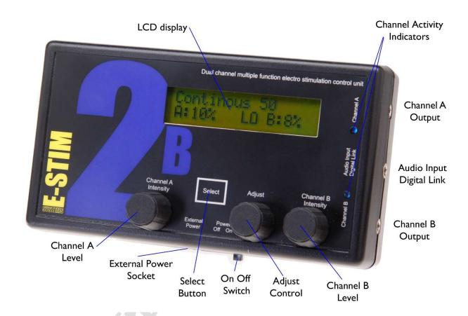
The 2B unit has five user controls. Each control allows the user to adjust a particular aspect of the output. It is the operation of the controls in combination that will allow the user to provide an effective electro-stimulation session.
