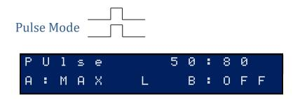
In pulse mode both of the outputs pulse on and off together. The adjustment control allows the user to adjust the pulse rate (how quickly they pulse on and off) and is adjustable from 2 to 100. Higher numbers indicate a faster pulse rate. The second value on the display, is the pulse feel, this allows you to adjust the sensation of each individual pulse, from soft to spiky, with values from 1 to 100.
