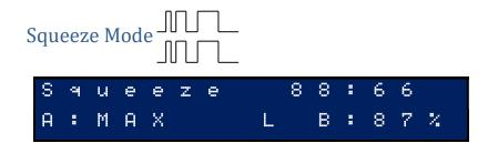
The pulse rate increases and then drops to nearly continuous producing a synchronised 'squeeze' sensation. Both Channel A and Channel B pulse at the same rate. The adjustment control controls how fast the pulse rate goes up or down with values from 10 to 100. The second value, is the pulse feel, that allows you to adjust the sensation of each individual pulse, from soft to spiky, with values from 1 to 100.
